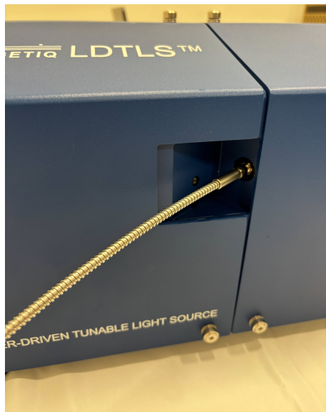
Figure 10. Connecting Output Fiber
