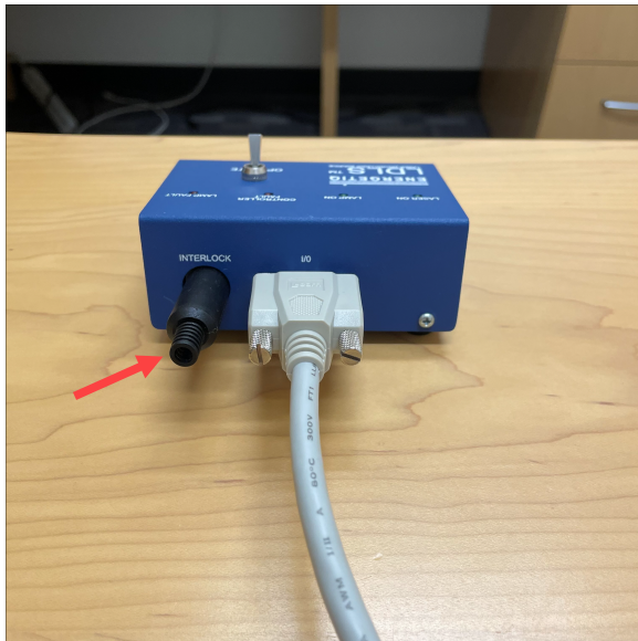
Figure 12. Inserting the Interlock Jumper Plug
