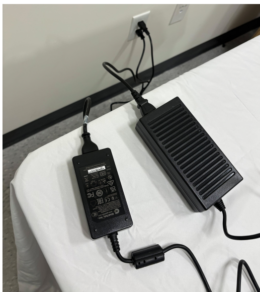
Figure 18. Plugging Power Supplies into 120VAC Outlets
