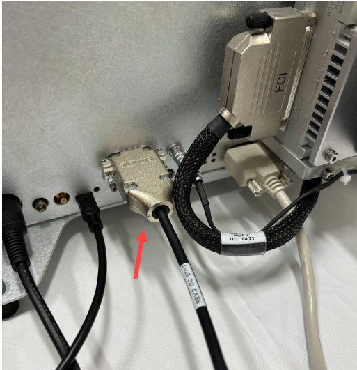
Figure 16. Connecting to Lamp Head Controller Port
