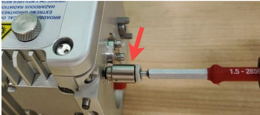
Figure 25. Reinstalling the Purge Fitting
