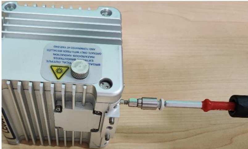
Figure 23. Removing the Purge Fitting
