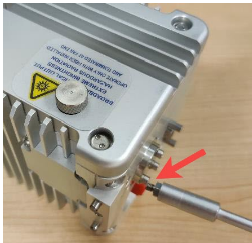
Figure 24. Removing the Flow Restrictor
