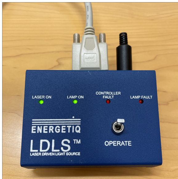
Figure 31. LAMP ON LED Illuminated
