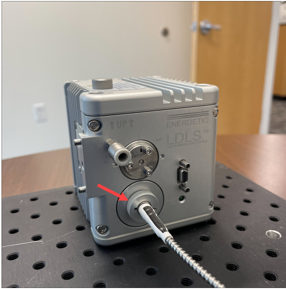
Figure 12. Connecting the Laser Fiber Optic Cable to Lamp Head
