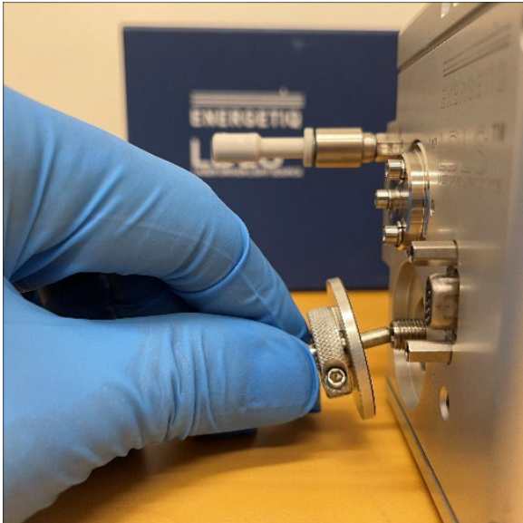
Figure 10. Inserting the Laser Fiber Optic Cable
