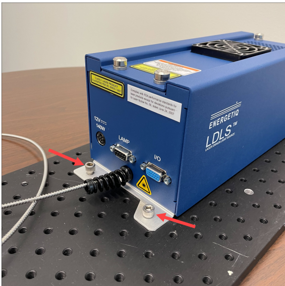
Figure 13. Mounting the LDLS Controller
