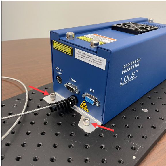
Figure 13. Mounting the LDLS Controller
