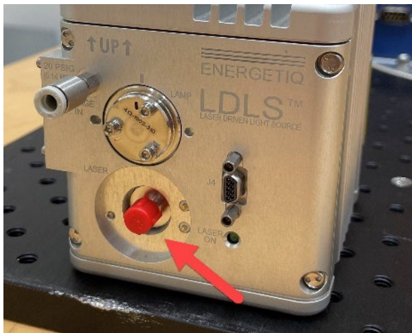
Figure 9. Removing the SMA Cap
