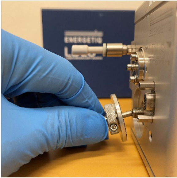
Figure 10. Inserting the Laser Fiber Optic Cable
