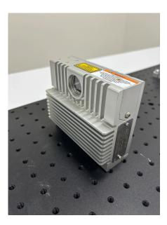
Figure 8. Removing the Lamp Output Window Covers
