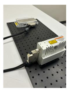
**Figure 10. Connecting the Interconnect Cable**
