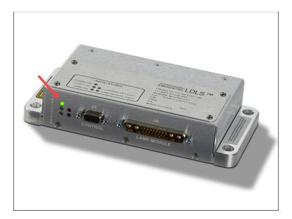
Figure 16. LDLS Controller "POWER ON" LED Illuminated
