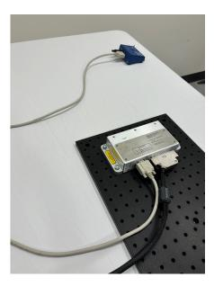
Figure 11. Connecting the I/O Cable to Remote Control
