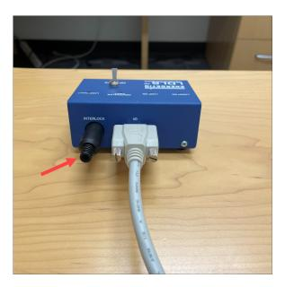
Figure 12. Inserting the Interlock Jumper Plug
