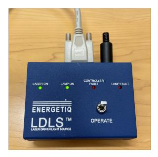
Figure 18. LAMP ON LED Illuminated
