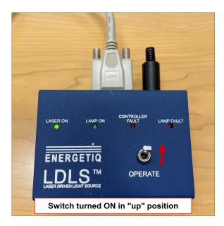
Figure 17. LASER ON LED Illuminated
