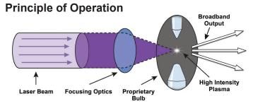
LDLS technology utilizes a laser to create an extremely small, high-brightness plasma with a broad spectral range.
