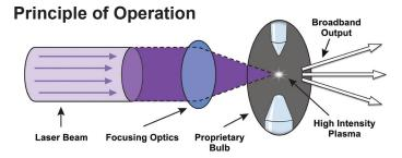
LDLS technology utilizes a laser to create an extremely small, high brightness plasma with a broad spectral range.
