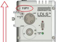
important for the EQ-99X-FC as it must be mounted with the output fiber optic connection on top. The plasma moves slightly depending on gravity and the precision ellipsoidal coupling optics in the EQ-99X-FC have been adjusted at the factory to optimize output in that particular orientation.
