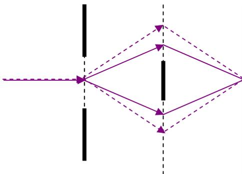
**Fig. 5.** Achromatic behavior of the two-grating interferometer. Dashed line represents a longer wavelength.
