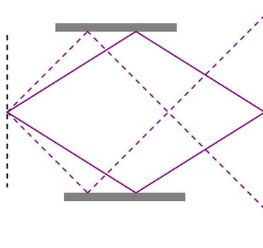
**Fig. 6.** Schematic of grating beam-splitter and two-mirror combiner configuration. This is equivalent to the Talbot prism combiner configuration. Each color represents a different wavelength. The dashed lines simply represent a different point in the field. Note that the requisite zero-order stop is not shown.
