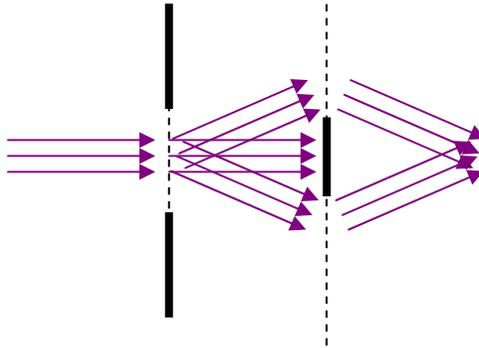
**Fig. 2.** Schematic of the two-grating interferometer. A second grating is used to recombine the beams separated by amplitude division from the first grating.
