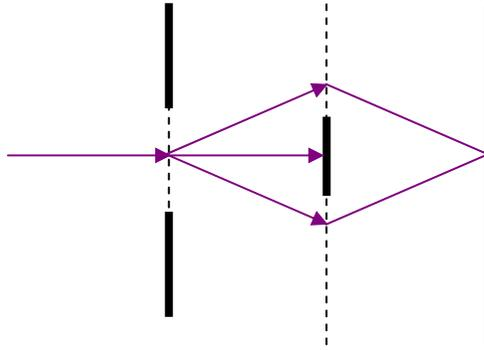
**Fig. 3.** Assuming the interference plane is properly chosen, the two grating interferometer interferes beam with zero shear.
