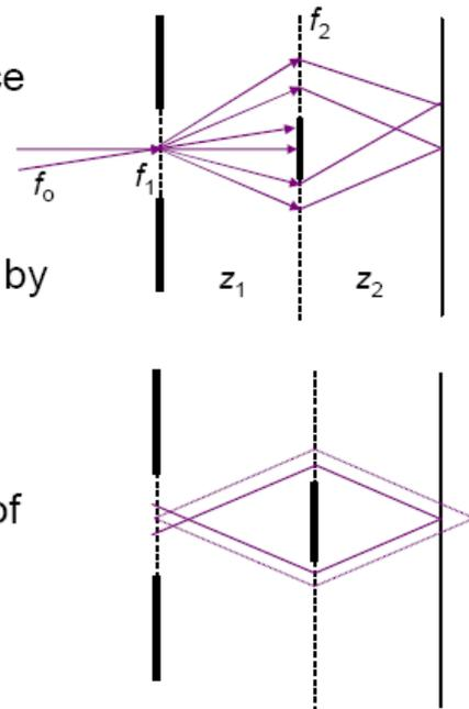
Figure 9: A two-grating broad-band interference device. (Courtesy Patrick Naulleau)
